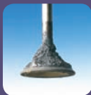
DIRTY INTAKE VALVE
